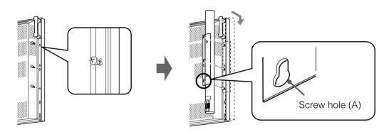
3. Tighten the mounting screws firmly with phillips screwdriver.
